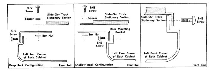
Fig. 6-4. Rack rails tapped for 10-32 machine screws.
