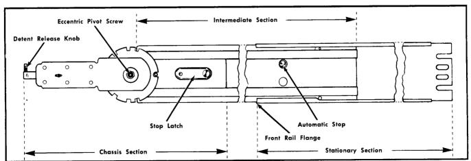
Fig. 6-3. Slide-out track assembly.
