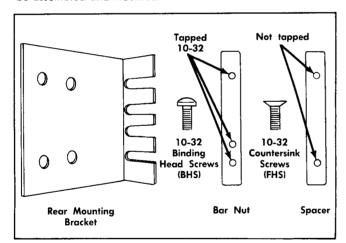
Fig. 6-1. Small mounting-hardware components.
