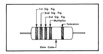
Fig. 3-2. Standard EIA color code for metal-film resistors.
