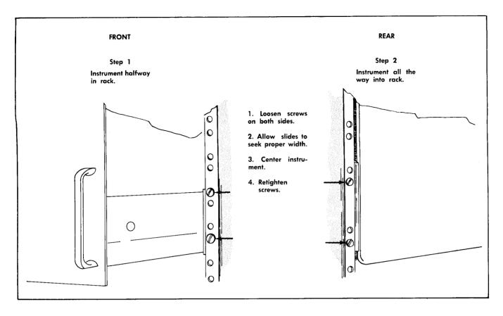
Fig. 6-7. Slide-out track adjustment for smooth operation.
