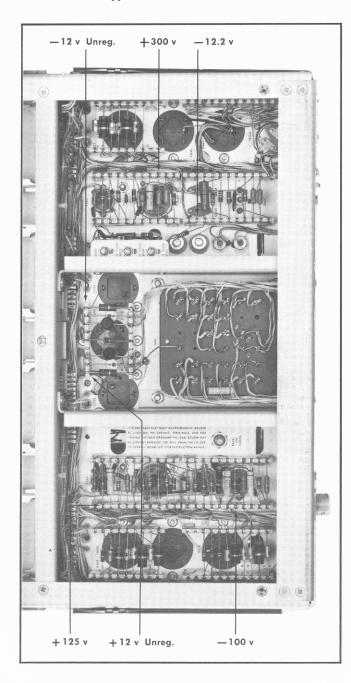
Fig. 4-1. Power supply test points.
