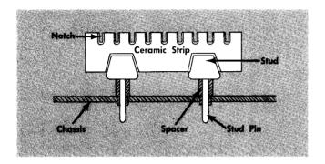
Fig. 3-1. Ceramic terminal strip assembly.
