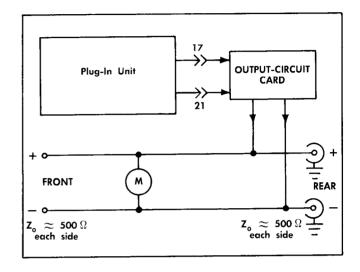
Fig. 1-1. Cathode-Follower Output-Circuit Card.
