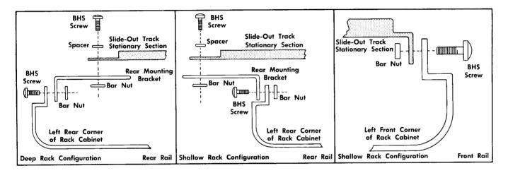
Fig. 6-5. Rack rails not tapped for 10-32 machine screws.
