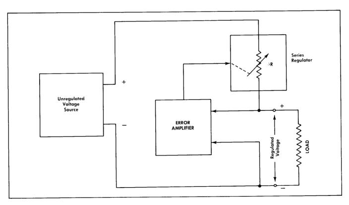
Fig. 2-1. Regulated supply principle.
