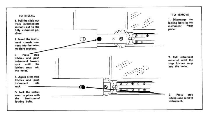
Fig. 6-6. Instrument installation and removal.
