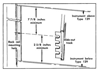
Fig. 6-2. Mounting hole location.
